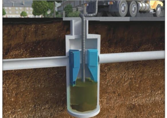
Fig.2 Maintenance is performed with a standard sump vac.
