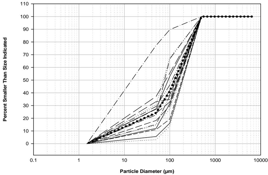
**Figure 9 Influent particle size distribution generated using serial filtration covering 500µm to 1.5µm particle size range; dashed line represents mean particle size distribution**
