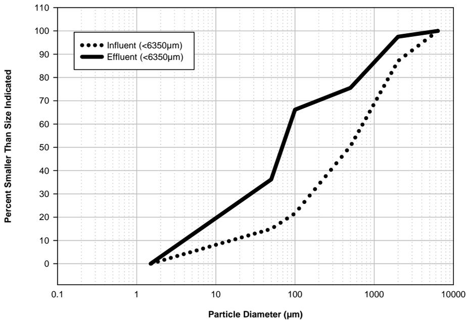
**Figure 10 Comparison of mean influent and effluent particle size distributions generated using serial filtration covering 6350µm to 1.5µm particle size range**
