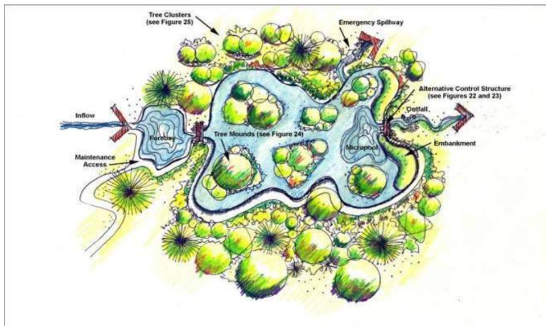
Figure 13.1: Plan View Constructed Wetland Basin
