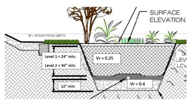
Figure 9.10. Typical Bioretention Section with Void Ratios for Volume Computations
