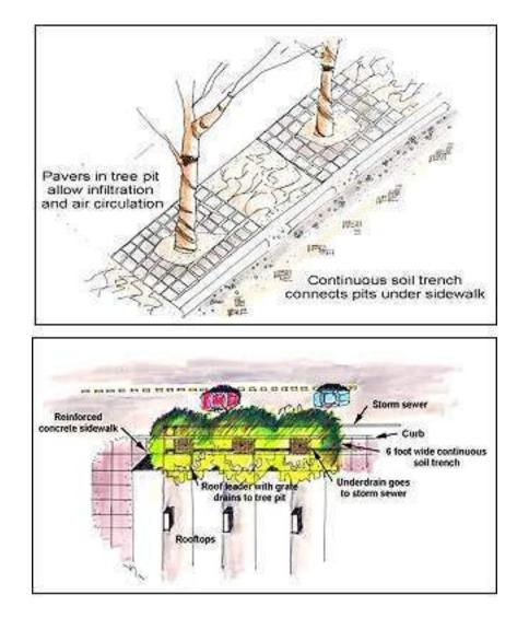
Figure 9-A.5. Expanded Tree Pit Details
