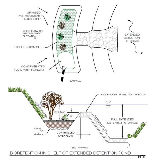
Figure 9.6. Typical Detail of a Bioretention Basin within the Upper Shelf of an ED Pond
