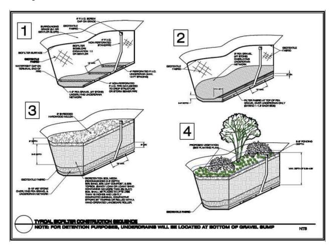
Figure 9.16. Typical Biofilter Construction Sequence
