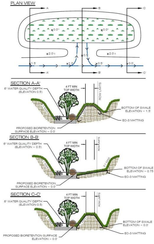
Figure 9.14. Typical Details for Off-Line Biofiltrattion
