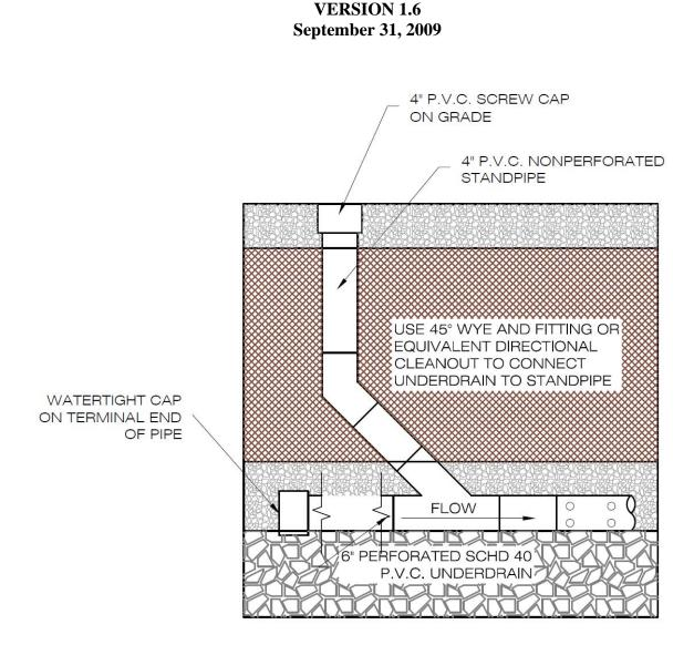
Figure 9-B.1. 4" P.V.C. Cleanout Detail
