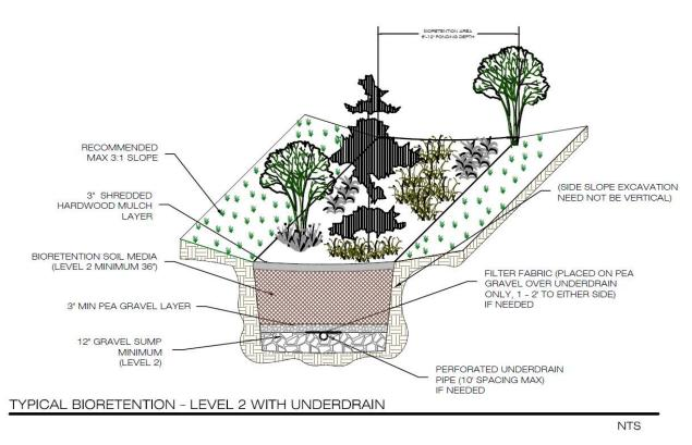
Figure 9.4b: Typical Detail of Bioretention Basin Level 2 Design
