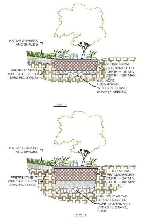
Figure 9.3B. Typical Micro-Bioretention Basin (Rain Garden) Level I and Level II – Section View:
