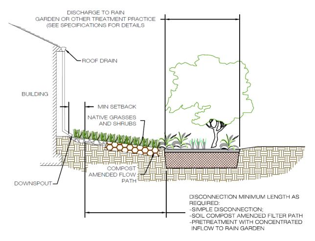
Figure 9.3A. Residential Rooftop Disconnection – Section View: (a) Simple Disconnection to downstream Raingarden; (b) Disconnection – Alternative Practice: Compost Amended Flow Path to downstream Raingarden
