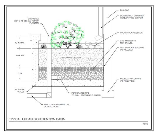
Figure 9-A.4. Stormwater Planter Cross-Section
