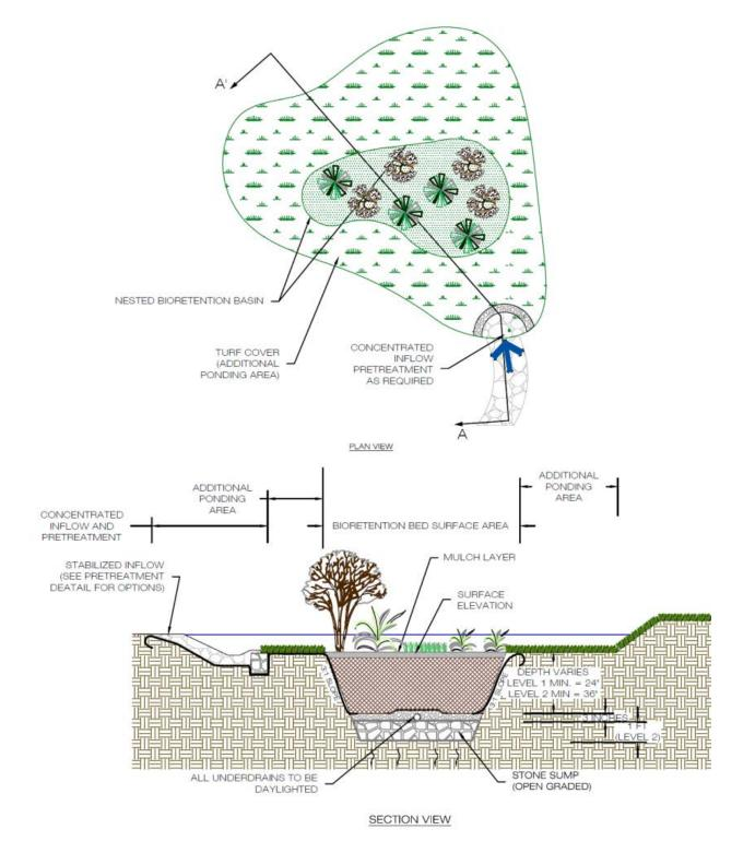
Figure 9.5. Typical Detail of Bioretention with Additional Surface Ponding
