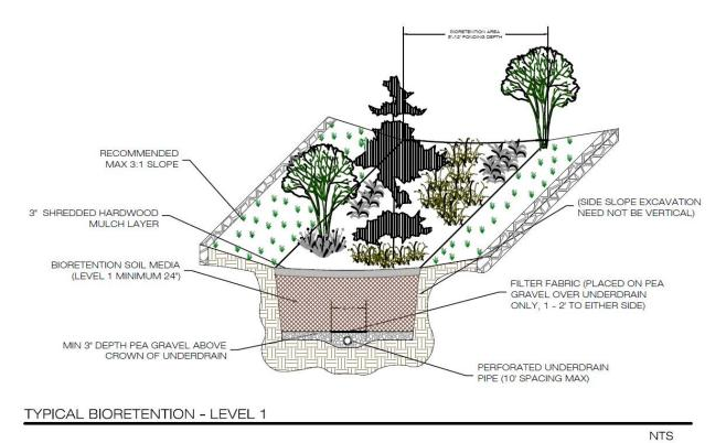
Figure 9.4a: Typical Detail of Bioretention Basin Level 1 Design
