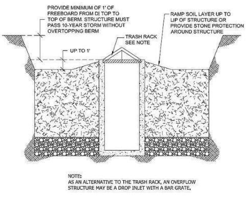
Figure 9.13. Typical Detail of how to prevent bypass or short-circuiting around the overflow structure
