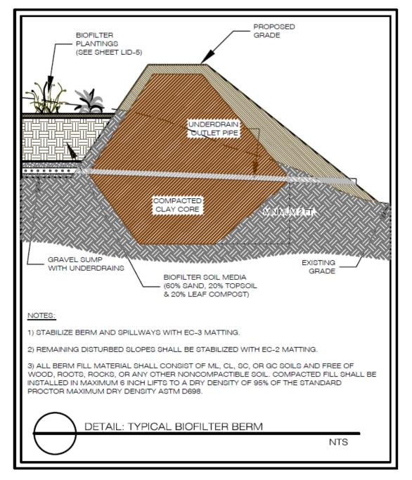
Figure 9-B.3. Typical Bioretention Basin Berm
